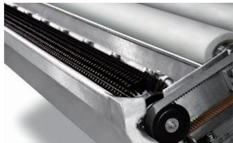
High speed belt cleaning system saves energy and cleans the belt more thoroughly. A tidy belt keeps the textile free from dirt.
